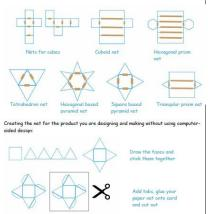
Chn use computer aided design (CAD) to explore the net shapes, remembering to include tabs on the edges (Purple Mash/Tinkercad). Chn experiment with the 2D nets to determine which shapes will make their 3D bridge stronger. Once they are happy with their refined plans, chn can print their net and use this as a template to begin to make the outline of their bridge.
